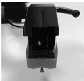
FIG. 7a: A CORRECTLY POSITIONED STYLUS
